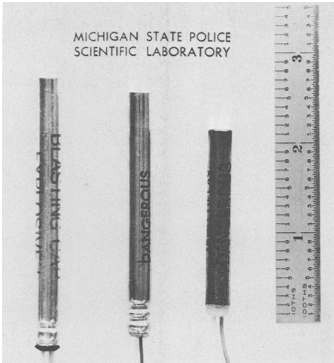
FIG. 2—Photograph of exterior configuration of Atlas, Dupont, and Hercules delay electric blasting caps.
